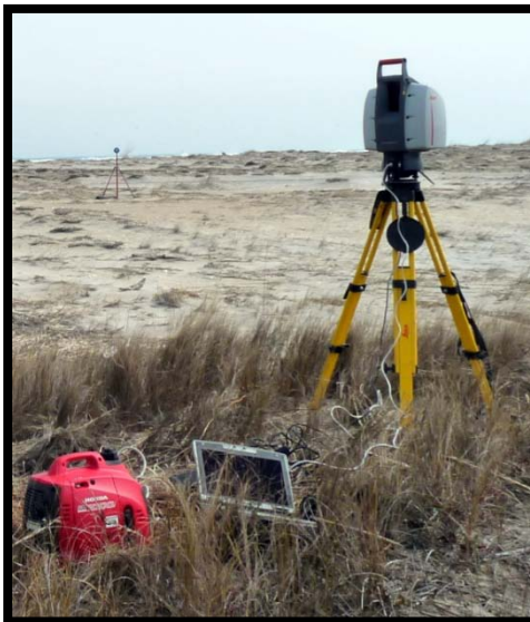
Figure 5. TLS setup. Landward extent of the overwash, February 2010.
